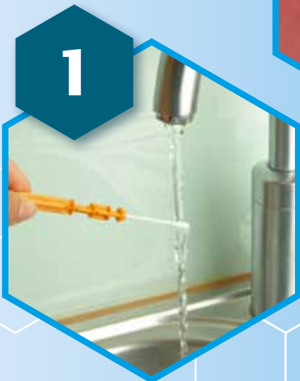
Moisten the swab with water (if the surface being investigated is dry).
