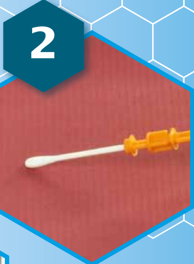
Wipe the swab over the object to be tested. Put the swab back in its cover and push it through both aluminium foils as far as the end stop.
