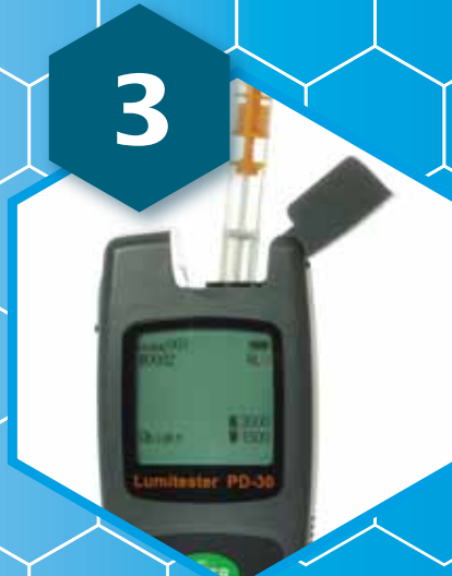
Shake the LuciPac Pen several times (vertical movement up and down) so that all of the liquid flows into the reaction chamber. As soon as the enzymes have dissolved, put the LuciPac Penrod in the device.
