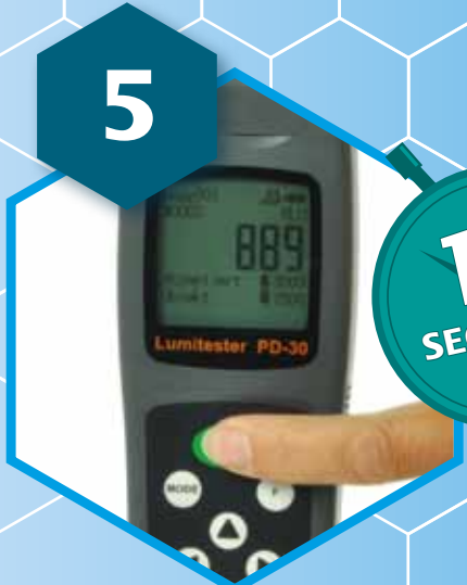
The measurement of invisible contamination is displayed as a numerical value in RLUs.
